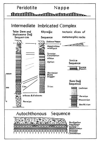
Fig. 5. Simplified stratigraphic sequences of the Lycian Nappes (from Graciansky 1968, modified).
