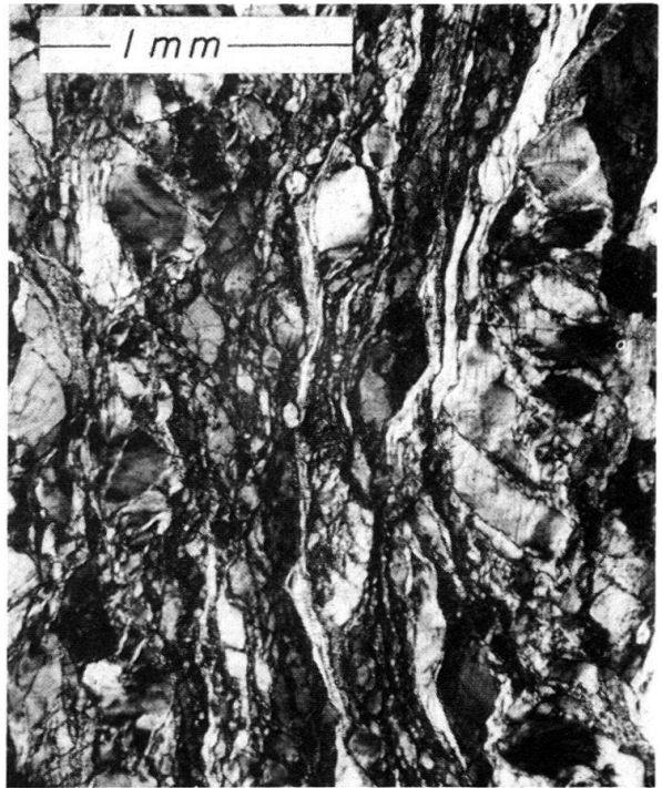
Fig. 12. Photomicrographs of mylonitic rocks close to the granite contact (1 km). a) Sci 308. Bergell granite N P. Cengalo. b) Sci 535. Tambo gneiss, V. Torta, 1,070 m, S. Vicosoprano. c) Sci 216. Gruf migmatite, Btta. Tegiola. d) VW 35. Experimentally deformed Cathedral peak quartz monzonite (compare Fig. 11a). Conditions: 900°C, 15kb confining pressure, 10^{-6} \text{ sec}^{-1} strain-rate, 60% shortening.
