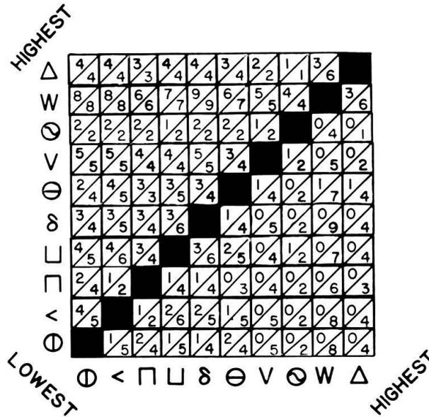
Figure 4. Revised matrix in which the ratio  $n/N$  has been rearranged so that all values greater than  $1/2$  are in the upper left part of the matrix. The lowest-highest sequence along the bottom and left side of the matrix now represent the most probable sequence of events.
