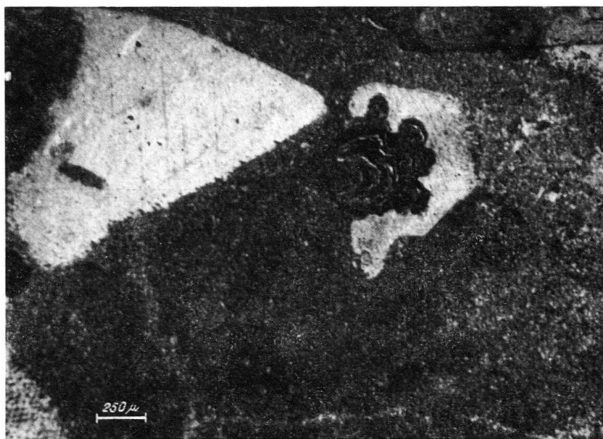
Fig. 10. Limonitic "cauliflower" structure cutting a crinoidal fragment. This shows the non-syngenetic origin of these structures. Crinoidal Limestone; parallel nicols.
