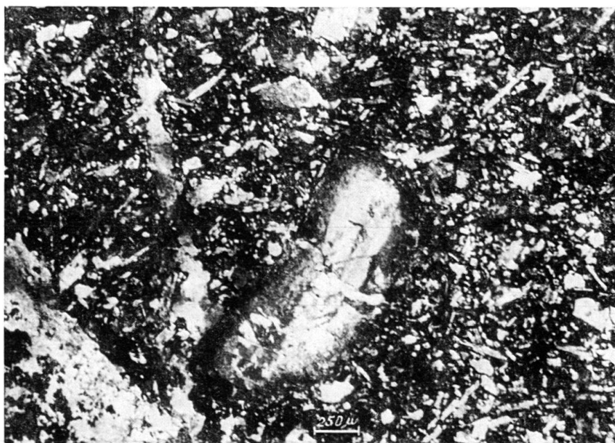
Fig. 7. Basaltic fragment with strongly altered plagioclase phenocryst. Parallel nicols.
