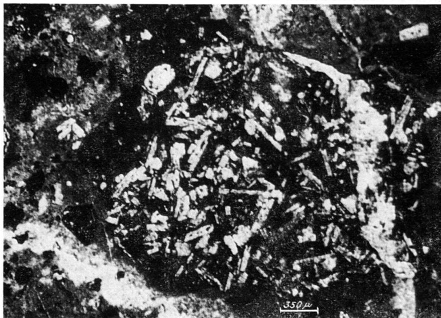
Fig. 4. Basaltic fragment with intersertal texture in impure red calcilutite. To left: few small fully limonitized grains. Parallel nicols.
