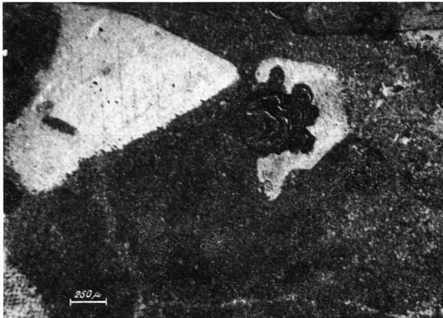
Fig. 10. Limonitic "cauliflower" structure cutting a crinoidal fragment. This shows the non-syngenetic origin of these structures. Crinoidal Limestone; parallel nicols.
