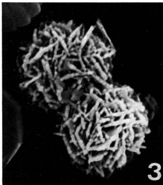
Fig. 3. Spherulitic aggregates composed of small platelets which constitute a second type of cement in the chalk. The flat surface of the aggregate in Figure 2 (arrow) was formed by close contact against a placolith shield. 12,600 $\times$
