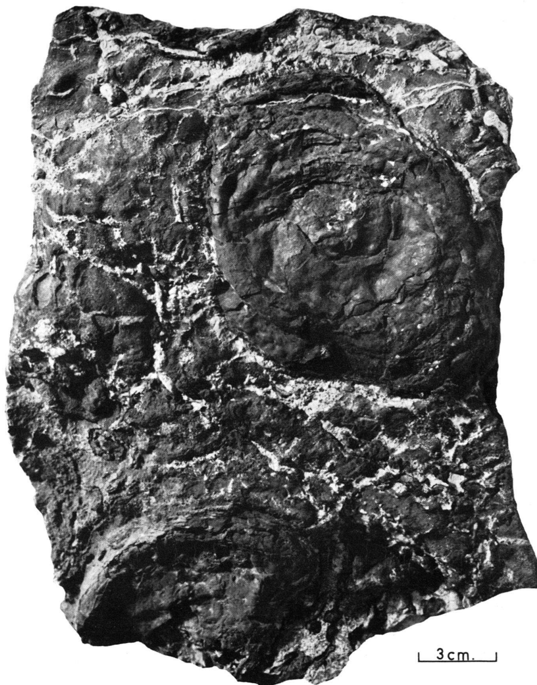
Fig. 6. Close-up view of the Monte Kumeta crust, showing fused "pancakes" of ferromanganese.
