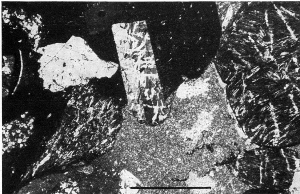
Fig. 13. Phenocrysts of sanidine and fragments of trachytic groundmass with flow structure set in ferruginous limestone. Crossed nicols. Monte Monaco, north-west Sicily. Scale bar = 1 mm.
