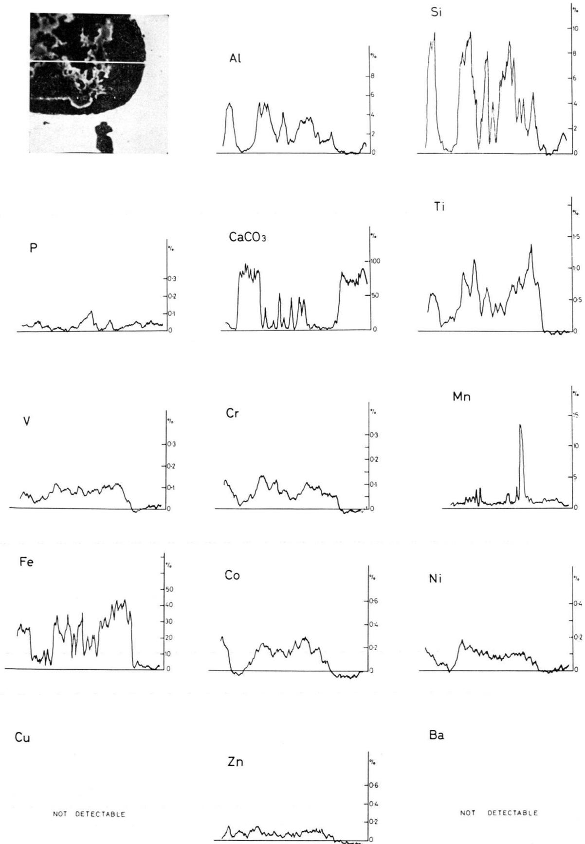
Fig. 14. Electron-probe microanalysis of an iron (chamosite-goethite-haematite) pisolith from the Toarcian of Rocce Maranfusa, western Sicily. Length of scan line = 375  $\mu$ .
