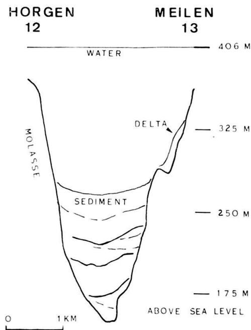
Fig. 2. Seismic profile traced directly from record. Vertical exaggeration is about 1:10. Solid lines may represent erosional unconformities.
