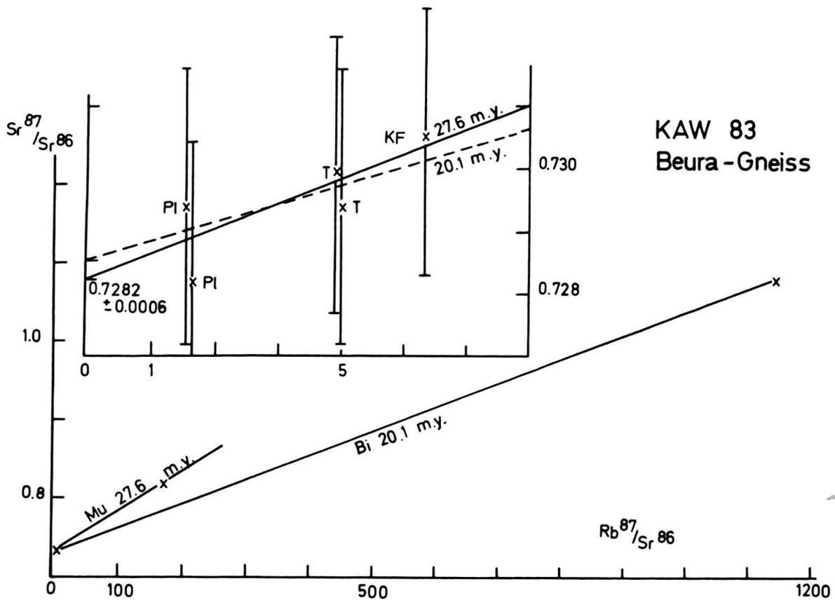
Fig. 7. Sr-evolution diagram of minerals and total rock from the Beura gneiss: T = total rock, Pl = plagioclase, KF = K-feldspar, Mu = muscovite and Bi = biotite.
