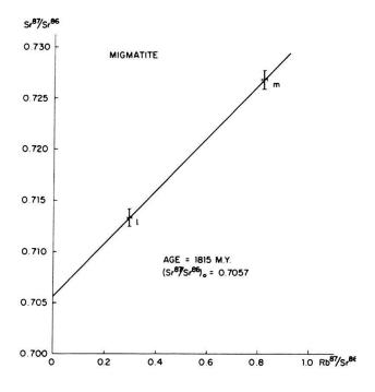
Fig. 5. Isochron plot for migmatite.
