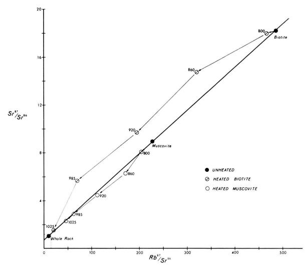
Fig. 2. Isochron plot of unheated and heated mica samples from the Prosperous Lake Granite. The numbers refer to the temperature (°C) of heating.
