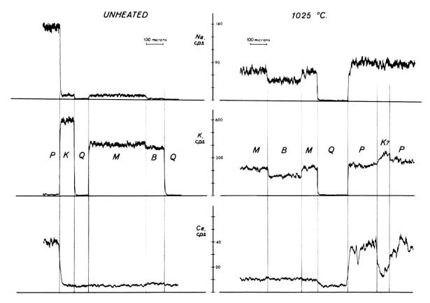
Fig. 9. Electron microprobe scans recording Na, K and Ca response from sections of the Prosperous Lake Granite heated to 1025 °C and unheated. P = plagioclase, K = K-feldspar, Q = quartz, M = muscovite and B = biotite.
