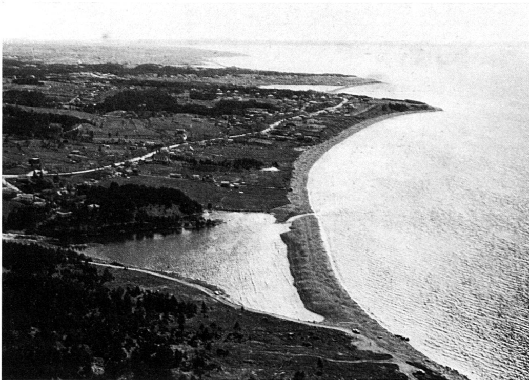
Fig. 20. Continuous gravel beach damming several lagoons along its course. Stone supply comes from glacial drift, which is exposed to wave erosion along the headlands and covers the bedrock in the whole area shown. The drift area beyond the lagoon in foreground is interrupted by two zones of flat solifluction and / or alluvial material, which were probably adjusted to a slightly raised sea level.
