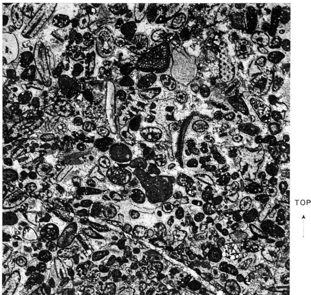
Fig. 6. Schrattenkalk: dasyclad algal lime grainstone . The grains are mainly worn fragments of the dasyclad alga Salpingoporella mühlbergii (Lorenz), with a few mollusc and crinoid fragments and worn benthonic forams such as miliolids and orbitolinids. The grains are coated by acicular drusy cement similar to that of modern beach rocks. This rock has probably been intermittently out of water. Environment: normal marine, high energy bar complex. Section No. 2, Habernlegi, Acetate peel, 10 \times .
