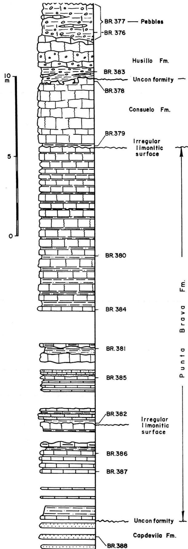
Fig. 65. Columnar section of the Punta Brava, Consuelo and Husillo formations, quarry east of Punta Brava.
