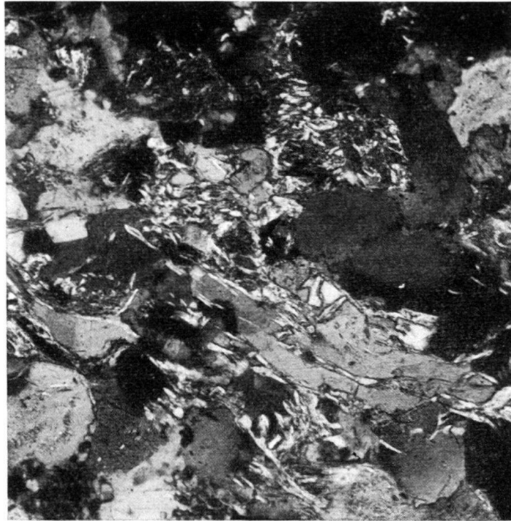
Fig. 6. Sandstone with quartz-regeneration structure, complicated by blastesis effect and linear segregation (quartz and muscovite). Western Verkhoianie ( P_1^1 ) IV zone. Magn. 90, 2 nicols.
