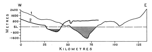
Fig. 2. Profils 1:1250000: (1) across G. of Aqaba in Lat. 28° 30′ N, and (2) across the Dead Sea in Lat. 31° 30′ N. (Vert. Exaggeration=8)
