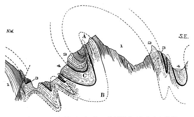
Fig. 1. Section across the Marwies after Heim (Tafel III, Pr. 18). Scale 1:25,000. 1 = Valangien and Neocomien; 2 = Schrattenkalk; 3 = Gault; 4 = Seewerkalk.
