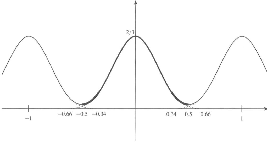
Fig. 3 Periodic signal  $s_{4A}(t)$  illustrating the aliasing effect with  $p_{4A}(t)$  highlighted in bold line. The extra-bold lines correspond to the aliased region that is behind the excess term  $\epsilon$  causing the sudden break in  $S_8$ . In this plot,  $\alpha = 0.33$ ,  $\delta = 0.08$ , and the vertical axis is scaled by  $1/\alpha^3$ .
