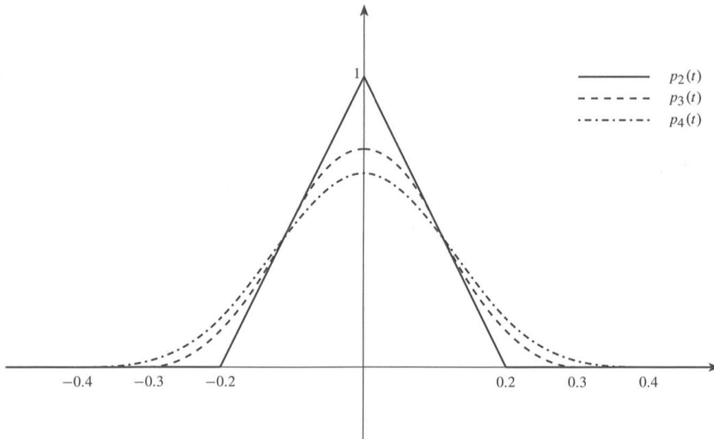
Fig. 2 Base pulses  $p_2(t)$ ,  $p_3(t)$ , and  $p_4(t)$  (respectively scaled by  $1/\alpha$ ,  $1/\alpha^2$ , and  $1/\alpha^3$ ) generated by the successive self-convolution of the rectangular base pulse  $p_1(t)$  for  $\alpha = 0.2$ .
