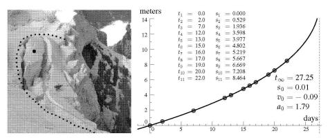
Fig. 4.6 Left: the Grindelwald hanging glacier with the surveying stake (Photo: M. Funk, from [7]); right: the data and the breaking off forecast
