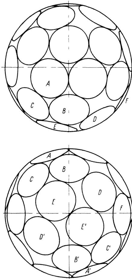
The symbol for this arrangement is 3, 3, 3, 3, 3, 3, 3, 3, 3, 3, 3. By successive approximation, the computed value of  $a_{33}$  obtained for this arrangement is  $36^\circ 15' 32''$ . In the following table, the latitudes and longitudes of one circle in each band are given. From these, one can verify by computation that adjacent circles do not overlap. For example, if  $BE$  is the angular distance between the centers of circles  $B$  and  $E$ , then
