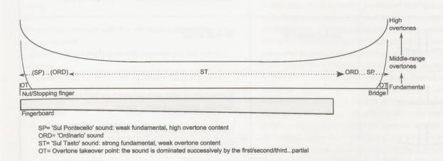
Figure 1: The overtone content for contact points along the whole string length. The cello string is represented by the horizontal line directly above the fingerboard. The curves above the string represent the number and relative loudness of the overtones that contribute to the resulting sound relative to contact point.
