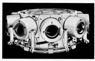
Poensgen Karussellanlage 10 Maschinen à 9, 15, 20, 30, 40, 50 kg pro Maschine
