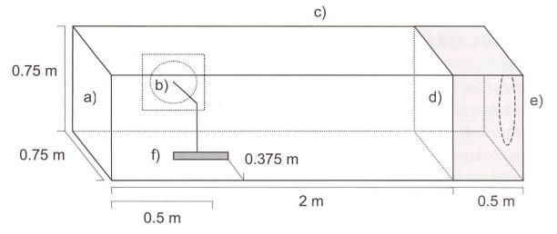
Fig. 1. Wind tunnel. a) coarse net and active carbon filter; b) hole to brace the experiment place outside the tunnel, closed with PVC; c) front part of the wind tunnel made of perspex; d) coarse and fine net spread in front of the motor, back part out of metal; e) motor; f) detailed sketch of the experiment place, round platform in the middle, surrounded by water, two wires installed to allow spiders to balloon; g) holding device for experiment place.
