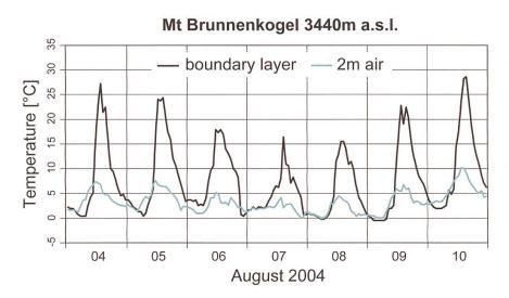
Fig. 5. Diurnal course of the boundary layer temperatures on soil surface (in shade) and air temperature at 2m height on Mt Brunnenkogel from 4<sup>th</sup> to 10<sup>th</sup> August 2004.
