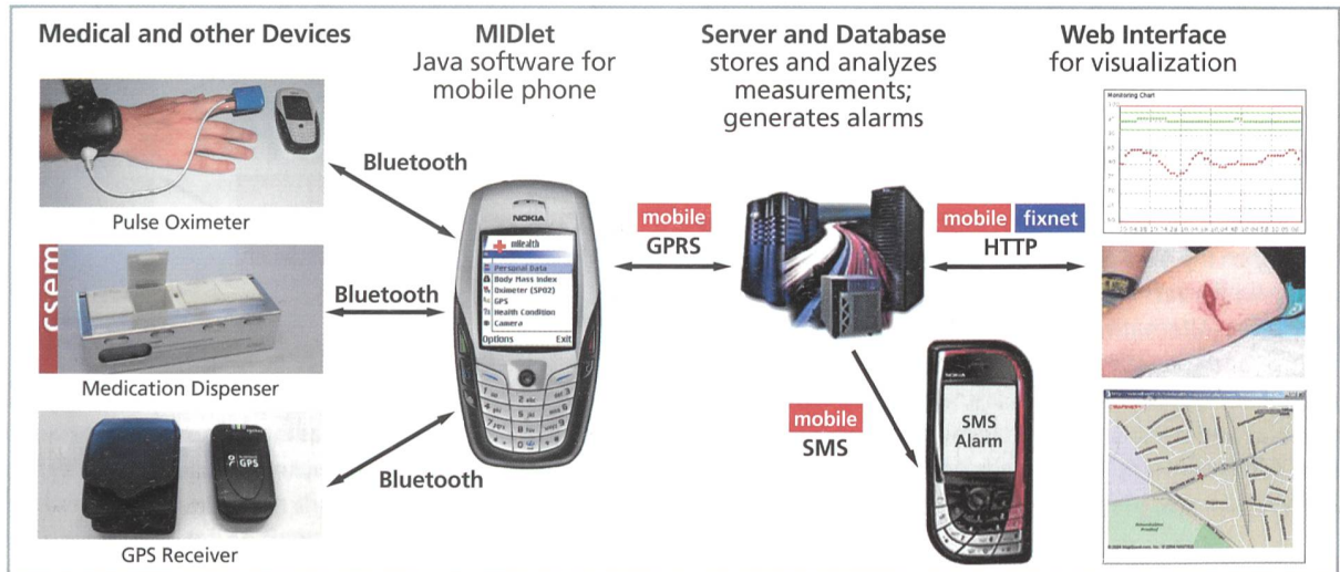
Fig. 3. Mobile health prototype. The mobile phone is used as normally for calls and messages, and, additionally, for connecting medical devices and for running the user interface for health services. The oximeter measures blood oxygen level and heart rate. The medication dispenser (courtesy of CSEM) controls taking of medicaments. The GPS receiver determines the geographic location. Measurements are forwarded via the mobile phone to a server and can be viewed by medical professionals in a Web Interface on a PC or mobile phone. Rules for sending automatic alarms via SMS can be defined.
