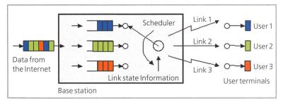
Fig. 1. Example setup for channel state dependent scheduling.
