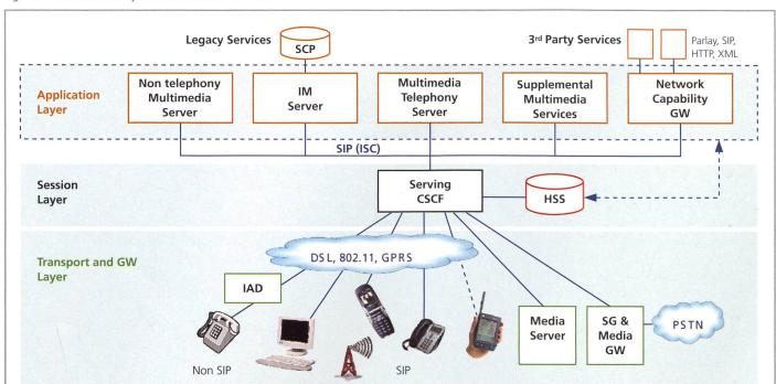
Fig. 1. IP Multimedia subsystem architecture overview.
