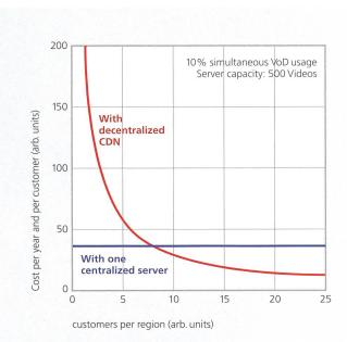
Fig. 4. VoD network and server cost per customer as a function of a regional customer-base (green cloud of fig. 3). VoD should begin with a centralised CDN. As soon as a critical amount of regional customers are reached, the decentralized CDN is the most economical solution.
