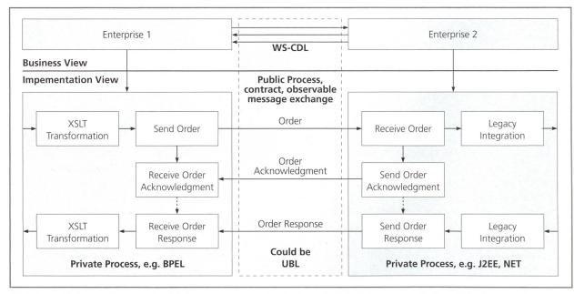
Fig. 1. A possible integration scenario with different process technologies and WS-CDL (Choreography Description Language) and UBL as common factors.
