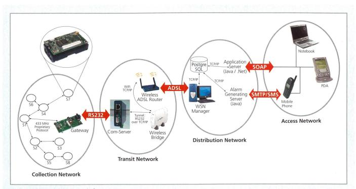
Fig. 3. Architecture of the demo platform.
