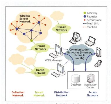
Fig. 1. General architecture necessary for WSN applications.
