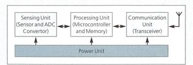
Fig. 2. Components of a sensor node.
