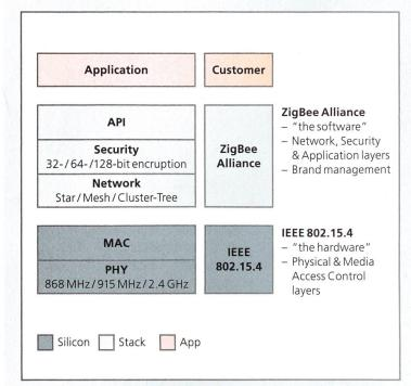
Fig. 4. ZigBee/IEEE 802.15.4 Protocol Stack. Source: Helicomm
