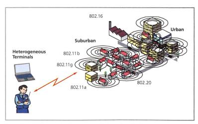
Fig. 2. The OBAN network will consist of a high number of micro-base stations based on WLAN-technology and randomly located in urban environments.
