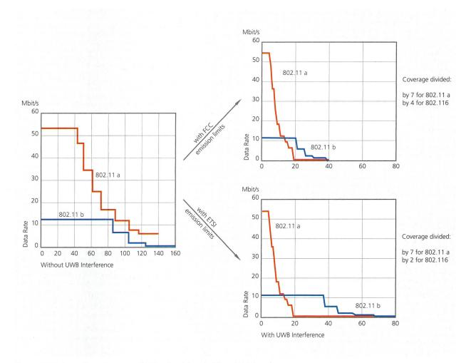
Fig. 2. Comparison of IEEE 802.11a and 802.11b, with and without UWB Interference.
