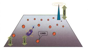
Fig. 1. In a GSM system, the base station location is high and inaccessible, whereas the mobile is lower and surrounded by UWB transmitters in office or personal communication devices. Therefore, the downlink is more critical regarding interference.
