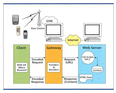
Bild 2. WAP-Funktionsmodell WAP 1.x (WAP: Wireless Application Protocol, GSM: Global System for Mobile Communications, WWW: World Wide Web, HTML: Hyper Text Markup Language, CGI: Common Gateway Interface, URL: Uniform Resource Locator).
