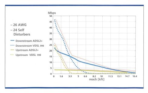
Fig. 3. ADSL2+ and VDSL Performance Comparison.
