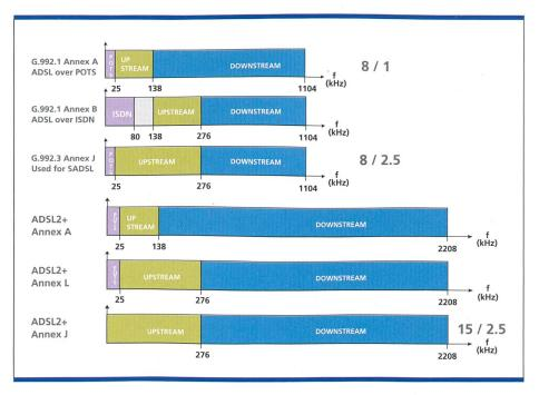
Fig. 1. The ADSL band plan.
