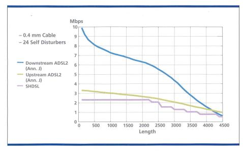
Fig. 4. SADSL and SHDSL Performance Comparison.
