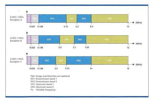
Fig. 2. The VDSL band plan.
