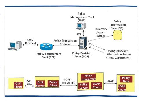
Fig. 1. Policy Based Networking Architecture.
