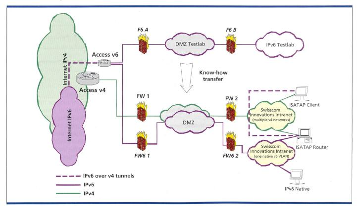
Fig. 3. Logical IPv6 network design at Swisscom Innovations.
