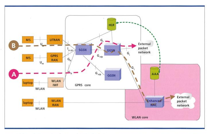
Fig. 2. Tightly coupled integration of WLAN and GPRS technologies.
