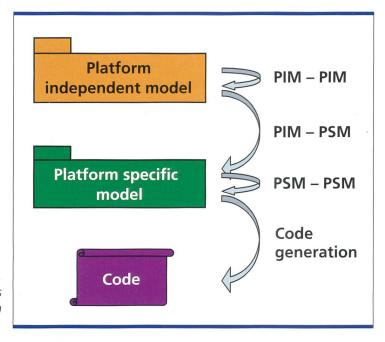
Fig. 2. Transformations on models in MDA.
