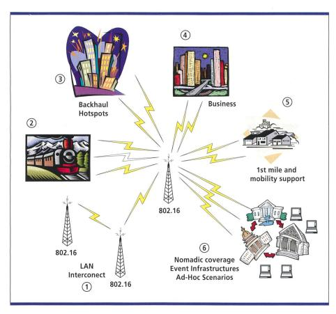
Fig. 3. Different scenarios enabled with 802.16a: ① LAN interconnection (connects the different locations of a company); ② Internet connectivity to trains (using 802.16e); ③ connecting Wireless LAN hotspots, as a cheaper alternative to leased lines or HDSL; ④ an alternative for connecting business offices; ⑤ an alternative for ADSL connections at home; ⑥ a flexible and quick solution for connecting temporary hotspots.
