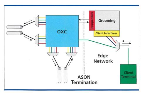
Fig. 3. One possible ASON node. It corresponds to a transparent optical node connected to the edge network through transponders, grooming and client interfaces.
