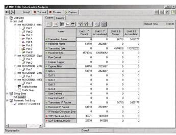
Fig. 7. The traffic counter feature has the ability to run a realtime graph function plotting two counters against an error condition.
