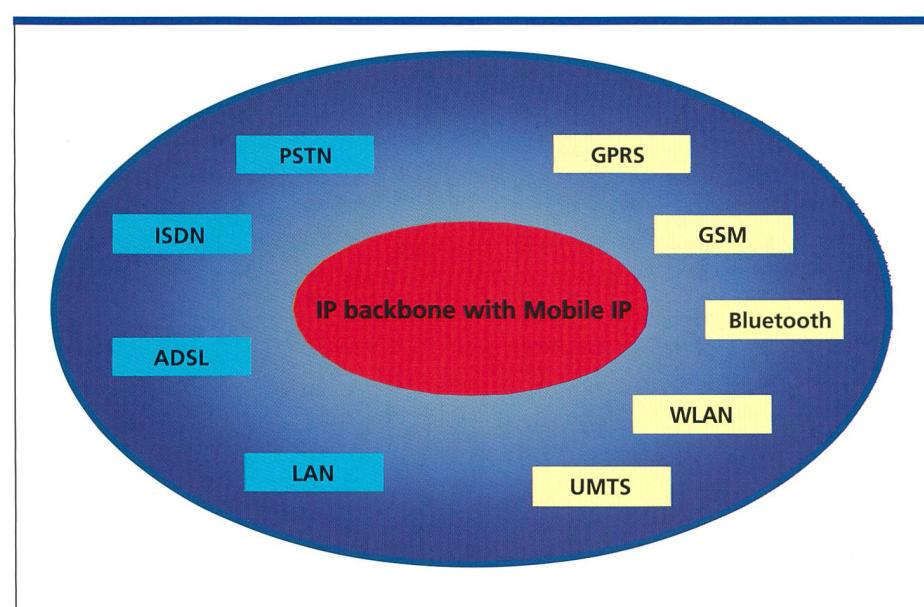
Fig. 4. Mobile IP integrates and complements different technologies.
