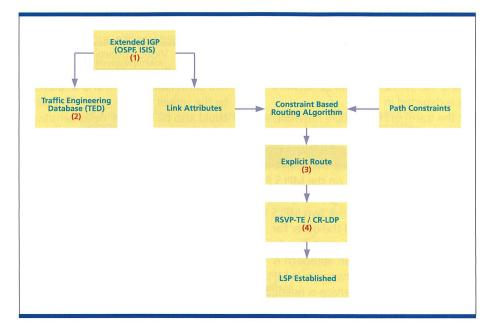
Fig. 1. Constraint-Based Routing operations.
