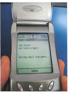
Fig. 4. A PeerDirectory instance running on Motorola A008.
