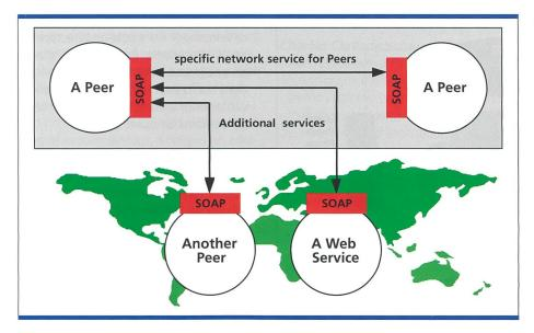
Fig. 2. A Peer with a SOAP interface can interact with any other SOAP enabled service. This increases flexibility and allows a Peer to participate in a bigger context.
