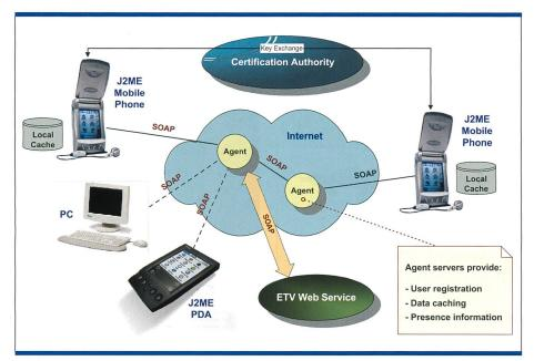
Fig. 5. The Software Architecture of the PeerDirectory application.
