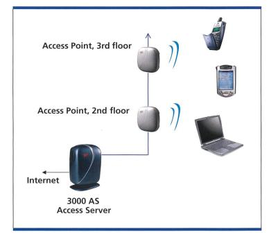
Fig. 1. Demo Platform architecture.
