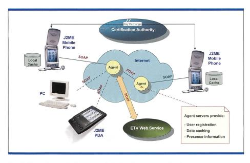
Fig. 5. The Software Architecture of the PeerDirectory application.
