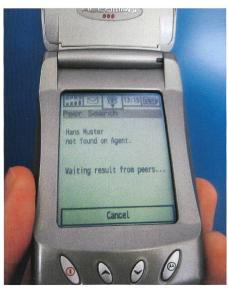
Fig. 4. A PeerDirectory instance running on Motorola A008.
