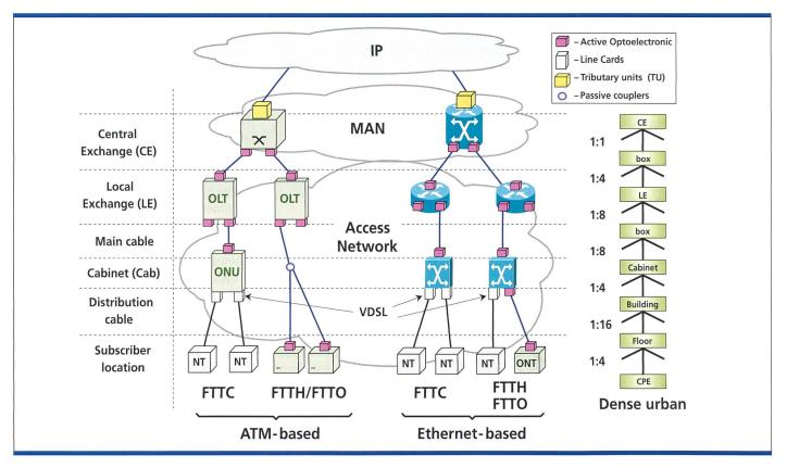
Fig. 4. The business case technology choice and architectural options. OLT: Optical Line Termination; ONU: Optical Network Unit; NT: Network Termination; ONT: Optical Network Termination; CPE: Customer Premises Equipment; MAN: Metropolitan Area Network.
