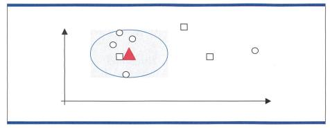
Fig. 6. Example of a k-nearest neighbour: The new item triangle is surrounded by a disc which contains four elements of class Circle, and one element of class Square. Therefore the new item will be classified in the class Circle.
