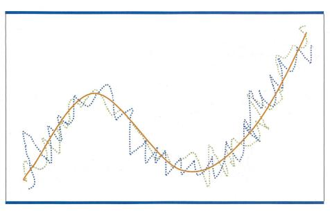
Fig. 3. The process of model building explained as a function regression task: The generalised model (red curve) acquired from the training data (blue curve) represents the important qualities in the test data (green curve). Good Generalisation Performance.
