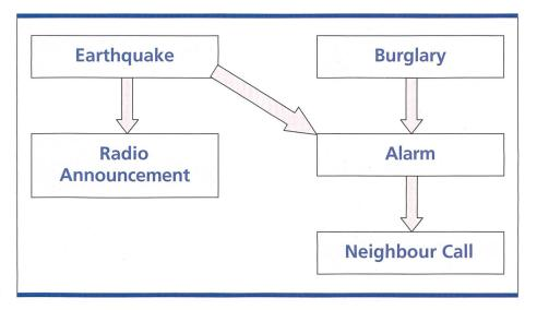
Fig. 7. Example of a Bayesian Network: Probabilities on each node are associated with this directed graph model. This means that, for example, given the state of Earthquake and Burglary, the probability that an alarm occurs is known.
