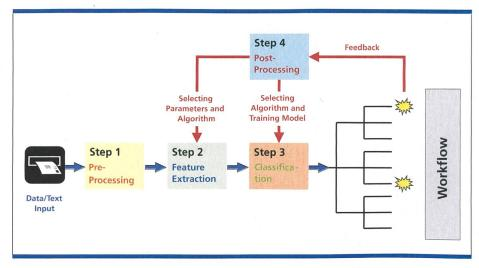
Fig. 1. The four steps of the automated Text Classification process.
