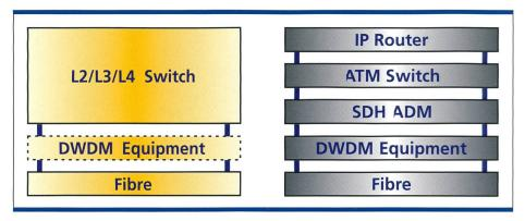
Fig. 2. Data network equipment: Ethernet-based (left) and SDH-based (right).
