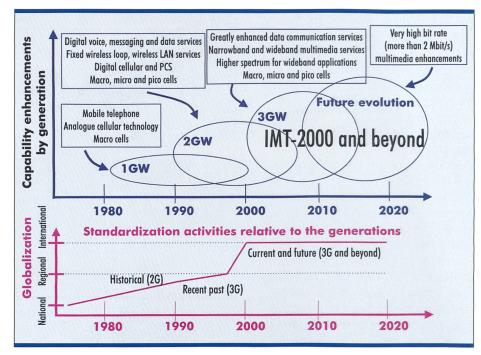
Fig. 5. Generations of terrestrial commercial wireless systems.
