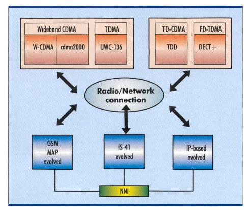
Fig. 3. IMT-2000 terrestrial radio interfaces.
